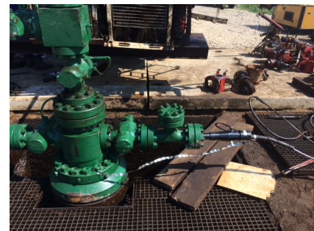
Cable packoff hardware can be used with a wellhead adapter (left), or it can be run through the annulus (right).
